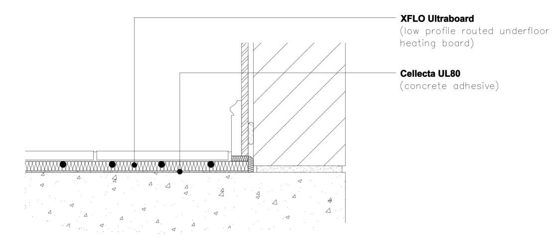
CELLECTA'S LOW PROFILE UFH INSULATION STRUCTURAL SEPARATING FLOOR — CONCRETE UNDERFLOOR HEATING BOARD UNDER TILE OR WOODEN FLOOR COVERING
